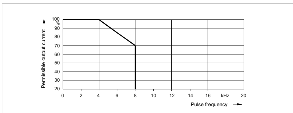
Figure 3-47 Frame size FSF: Output current as a function of the pulse frequency
